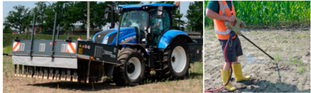
Figure 1. Picture of the Zasso XP300 Xpower (left) and Rootwave Pro (right) electric weeding devices.
